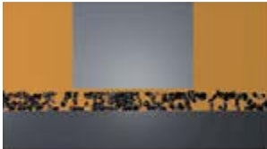
CONTAMINATION IN PRESENCE OF LARGE TOLERANCES
