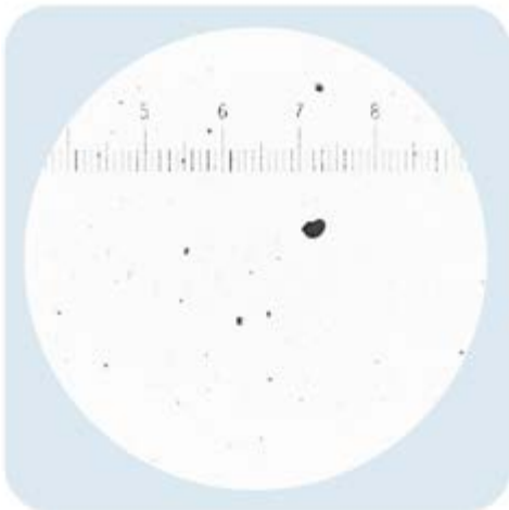
ISO 4406 Class 20/18/15 SAE AS4059 Table 1 Class 9 NAS 1638 Class 9 SAE AS4059 Table 2 Class 10A/9B/9C
