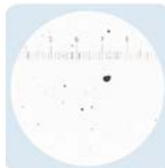
NAS 9 ISO 21/18/15 Typically new oil as delivered in oil tankers
