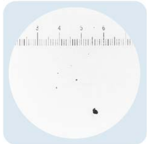
ISO 4406 Class 15/13/10 SAE AS4059 Table 1 Class 4 NAS 1638 Class 4 SAE AS4059 Table 2 Class 5A/4B/4C
