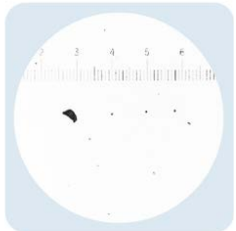
ISO 4406 Class 17/15/12 SAE AS4059 Table 1 Class 6 NAS 1638 Class 6 SAE AS4059 Table 2 Class 7A/6B/6C
