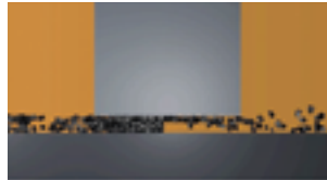
CONTAMINATION IN PRESENCE OF NARROW TOLERANCES
