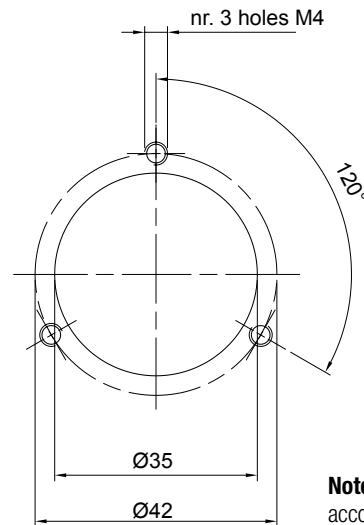
**Note:** Arrange the holes according to the position of the level indicator
