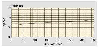
Bypass valve pressure drop
