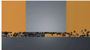
CONTAMINATION IN PRESENCE OF NARROW TOLERANCES
