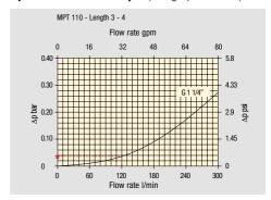
Filter housings  $\Delta p$  pressure drop. The curves are plotted using mineral oil with density of 0.86 kg/dm³ / 53.68 lb/ft³ in compliance with ISO 3968.  $\Delta p$  varies proportionally with density.
