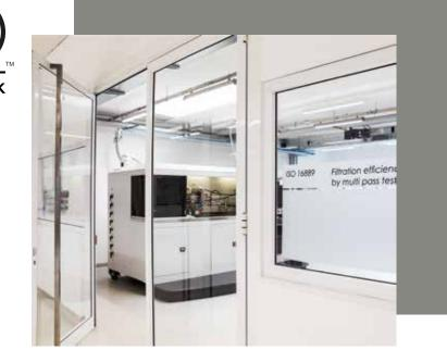
Supported by the latest technology, including scanning electron microscopes, MP Filtri's exhaustive testing programme is carried out with special emphasis on its comprehensive MULTIPASS analysis – which has been created in accordance with ISO16889. This method compares the amount of contaminant present upstream and downstream in the filter element – calculating the ratio of Beta filtration by the size of the particles and retention capacity.
