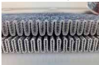
The Filter Media has absorbed water
