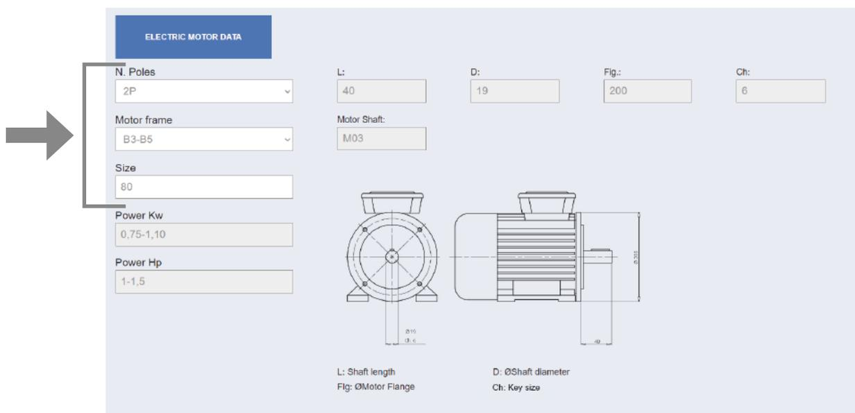
Once above data are input, fields related to motor sizes and technical drawing will appear, with data taken from the database, created from motor manufacturer official data.
