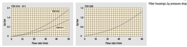
The curves are plotted using mineral oil with density of 0.86 kg/dm<sup>3</sup> in compliance with ISO 3968. ∆p varies proportionally with density.
