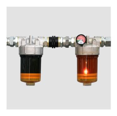
This new specific bench allowed tests to be carried out under different flow and temperature conditions for both in-line filters (e.g. FMM) and return filters (e.g. MPFX) up to 250 l/min. It is also possible to change the type of oil, verifying the potential characteristics of the filters under different operating conditions.
