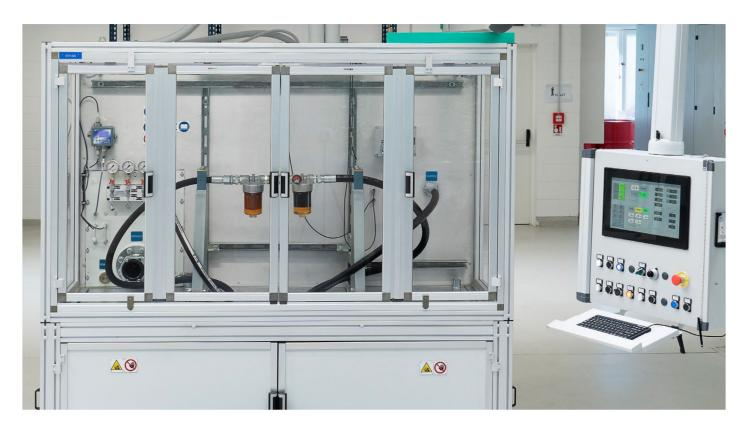
The specific hydraulic system and the instruments used are capable of measuring and recording the electrical potential generated when a filter is crossed by a flow of oil, measured in kV.
