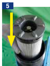
5 Insert the filter element into the filter body
