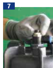
7 Make sure the air vent is closed
