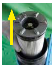
3 Remove the filter element
