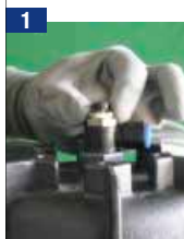
1 Loosen the air vent nut
