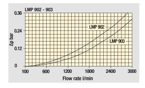
Bypass valve pressure drop
