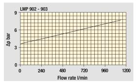
The curves are plotted using mineral oil with density of 0.86 kg/dm³ in compliance with ISO 3968. Δp varies proportionally with density.
