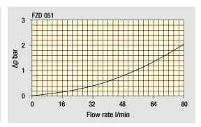
The curves are plotted using mineral oil with density of  $0.86 \text{ kg/dm}^3$  in compliance with ISO 3968.  $\Delta p$  varies proportionally with density.
