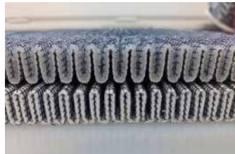
The Filter Media has absorbed water
